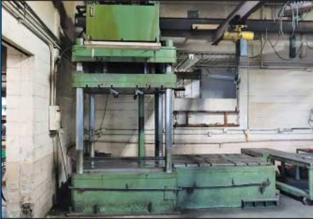
Inter-Continental Model 86-48-72-60-04 Sliding Bed Hydraulic Spotting Press
