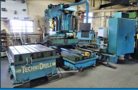
Techni-Drill Model 100-1.250-48-36-5A CNC Gun Drill
