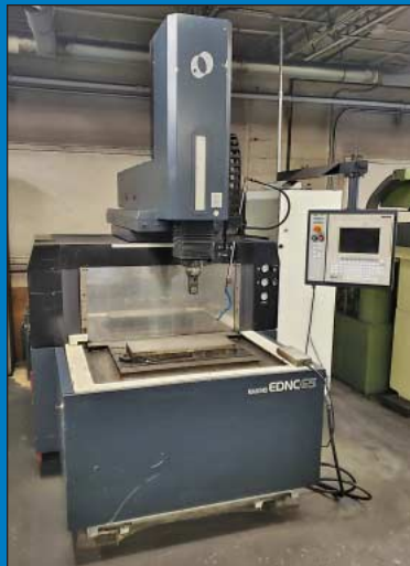
Makino Model EDNC-6 Die Sinker EDM w/ 4th-Axis Rotary Head
